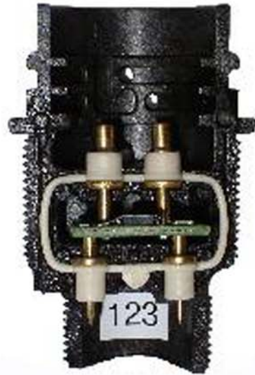
Individually addressed lamp holders
